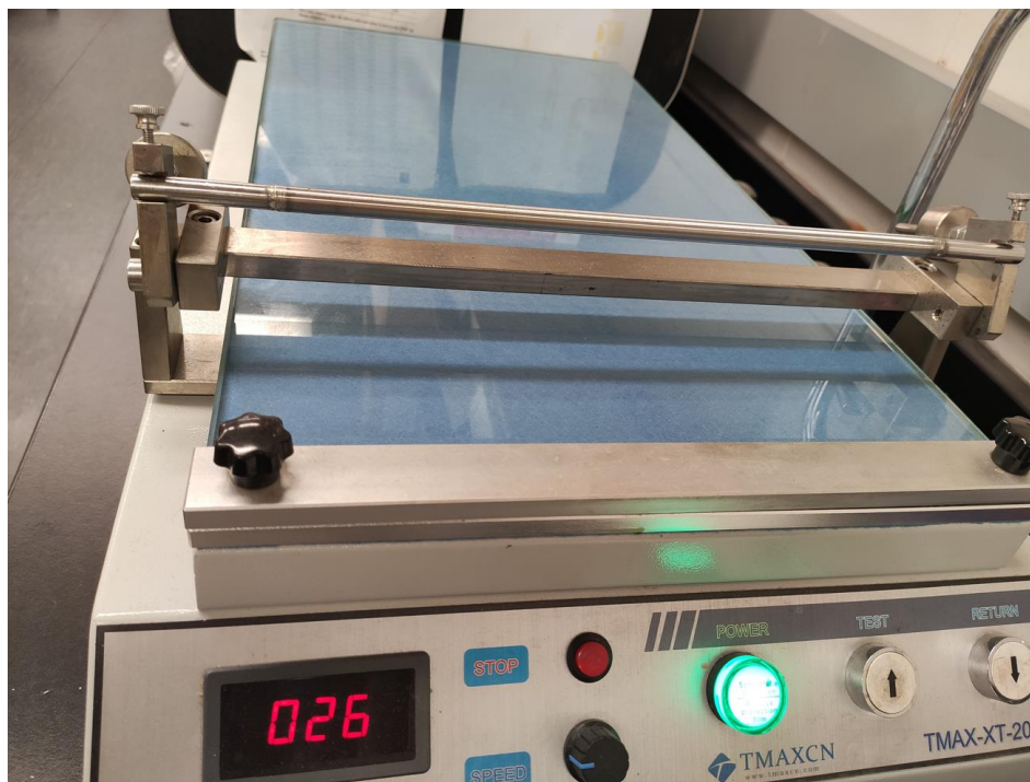
Figure 34 Mayer rod coating machine (TMAX-XT-200CA, Xiamen Tmax Battery Equipment Limited).
