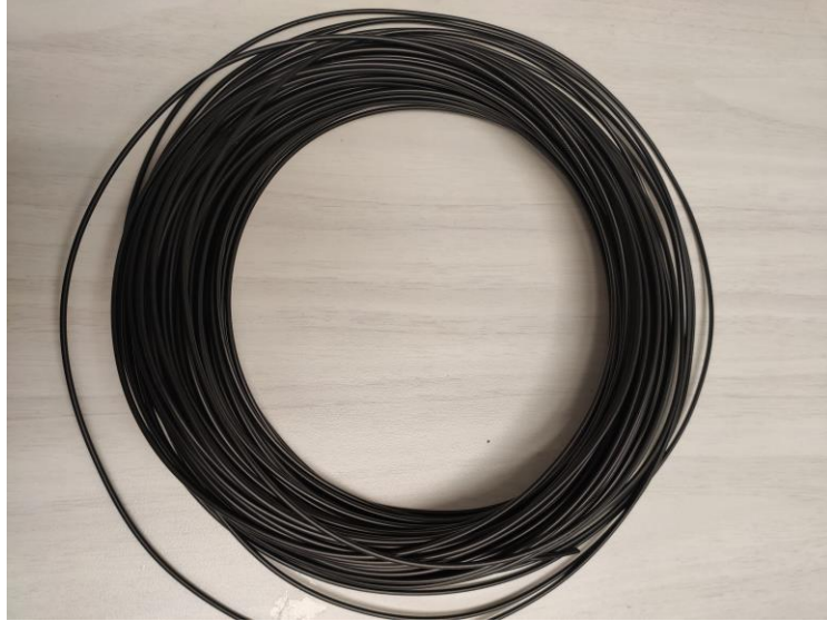
Figure 64 Prepared conductive PLA filament
