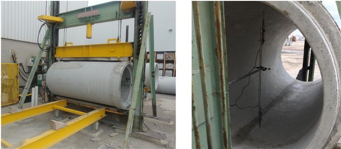
Figure 3.5-TEBT Setup (Left) and LVIT Setup (Right).
