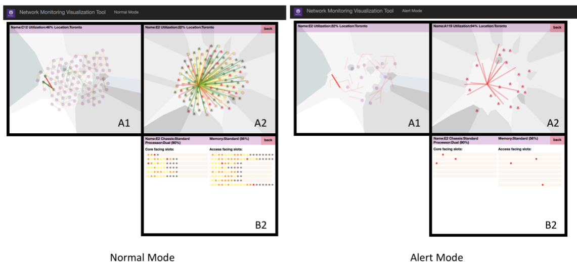
Figure 28: The comparison between the normal mode and the alert mode
