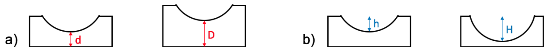
Figure 2.13 Instability is frequently treated by (a) increasing polyethylene offset d \rightarrow D , or (b) increasing constraint h \rightarrow H .
