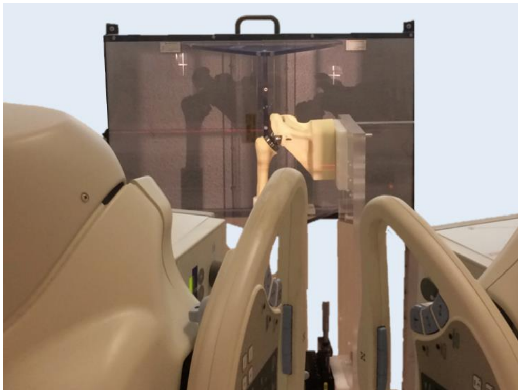
Figure 3.2 RSA setup for the shoulder phantom: the phantom is attached to a translation and rotation stage in front of a uniplanar calibration cage.
