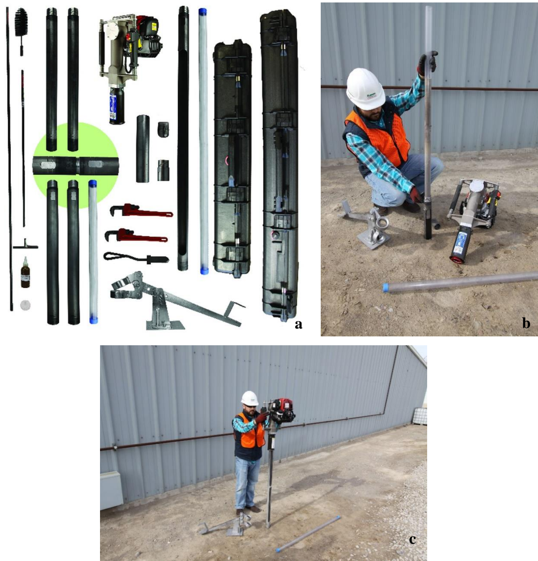
Figure 2.2. Images of the soil sampling kit used to extract soil cores on Pelee Island. A) Disassembled components of the sampling kit; B) assembly of the sampling kit; C) operation of the sampling kit. Figures retrieved from the AMS website (AMS 2019).
