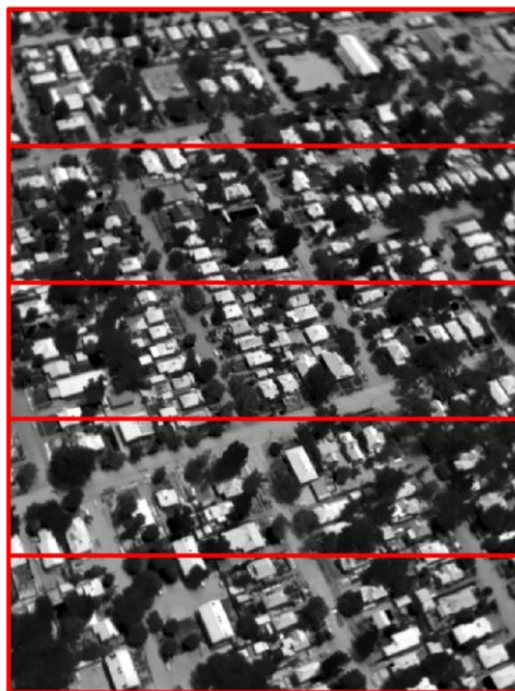
Figure 2.16 Thermal image with the five different atmospheric correction zones indicated by red boxes. The uppermost rectangle has the longest path length and thus the correction polynomial yields the largest corrections; the bottom most rectangle has the shortest path length and leads to smaller correction magnitudes (see e.g. Figure 2.16). The observer is East facing at a 45^\circ ONA.
