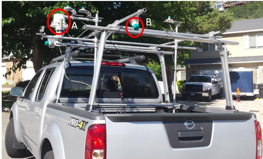
Figure 2.8 Truck mount and instruments. Label A shows the aspirated radiation shield that contains the humidity and air temperature sensors and B indicates the road-facing infrared radiometer. The FLIR T450 thermal imager is not shown but was positioned to view out the driver side rear window. The truck platform also includes incident shortwave, longwave, and PAR radiation sensors, a GoPro camera and a horizontally oriented infrared radiometer.
