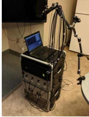
Figure 6.1: Picture of the TR-fNIRS system after setup at a long-term care facility
