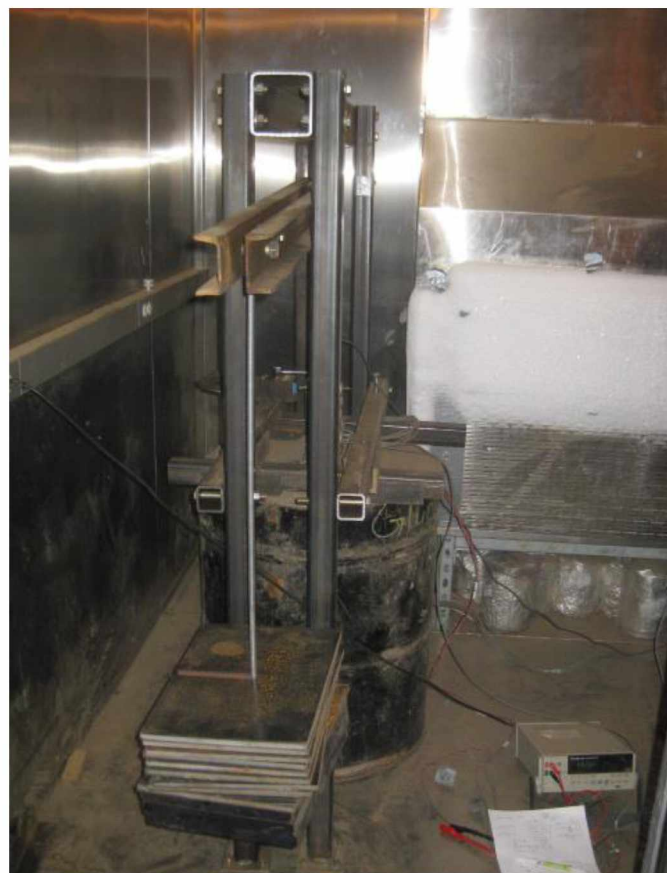
Figure A.18 Backfill the silt slurry into the annular space.
