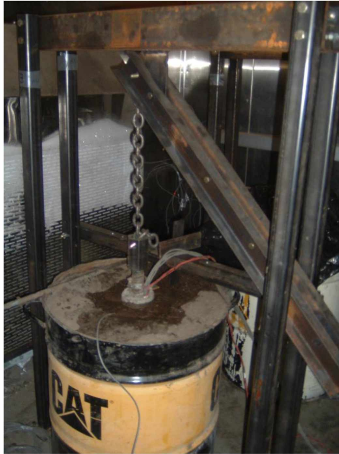
Figure A.16 The test anchor embedded in the unfrozen silt.
