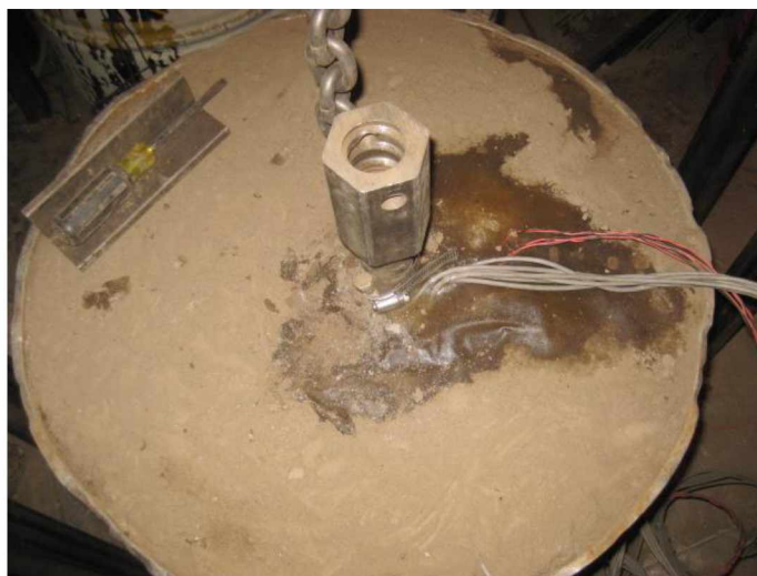
Figure A.17 Ice formed on the surface after the silt was frozen.
