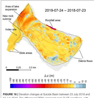
24 July 2019. The differenced DEMs represent post-GLOF conditions, with similar water levels in the basin (386 m in 2018 and 383 m in 2019). The colormap features a 5 m color spacing, except for the  $\pm 1$  m interval, which features a light gray tone. The black line delineates the maximum lake extent in 2019.
