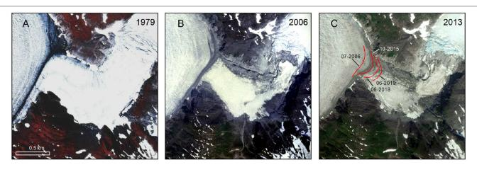
FIGURE 3 | Orthophotos from (A) 11 August 1979, (B) 3 July 2006, and (C) 28 July 2013, showing the rapid decay of Suicide Basin's ice cover. The red lines in (C) trace the position of the former middle moraine from 2006 to 2019, revealing several hundred meters of ice motion into the basin. The WorldView-2 image shown in (C) was processed by the Polar Geospatial Center (www.pgc.umn.edu, © 2013, DigitalGlobe, Inc.).
