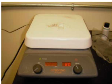
Figure 30: Preheat hotplate to 80°C.
