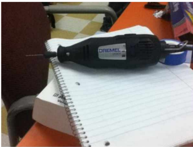
Figure 10: Dremel Model 200 with 1/32" Drill Bit (Robert Bosch Tool Corp., IL)
