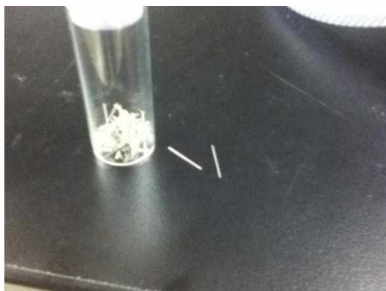
Figure 12: 0.025in Outer Diameter Stainless Steel Round-Tip Probe (itronx, Inc., CA)
