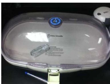
Figure 23: A large vacuum is used to eliminate the air bubbles that are created when the PDMS mixture is stirred and poured in the container.
