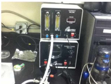
Figure 4: Harrick Plasma Plasmaflo PDC-FMG & Harrick Plasma Plasma Cleaner PDC-32G (Harrick Plasma NY)
