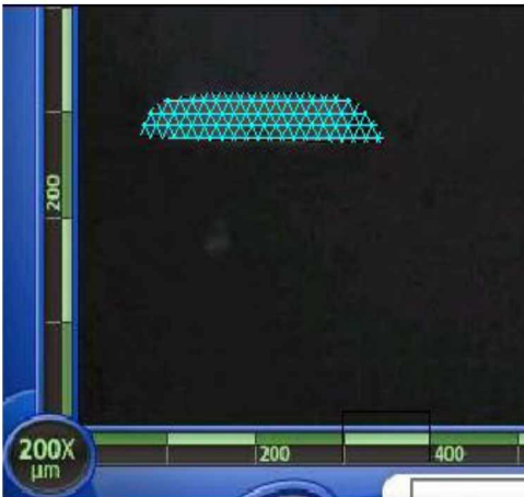
Figure 37: Cut of 1.25pt line width channel. The cross sectional area and perimeter were measured using AutoCAD area toolbar. A_c = 9909\mu\text{m}^2 P = 591\mu\text{m} .
