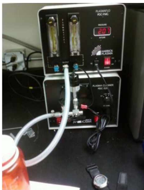
Figure 28: Adjustment of pressure is done by turning the knob attached to the chamber cap clockwise to reduce the pressure and counterclockwise to increase the pressure.
