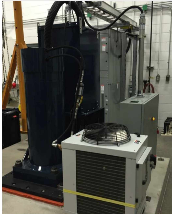
Figure 3.12. The Williams-Hatch 200 kW flywheel (large black cylinder) during testing and development at the ACEP Power System Integration Laboratory at the University of Alaska Fairbanks. Source: Alaska Center for Energy and Power, University of Alaska Fairbanks.
