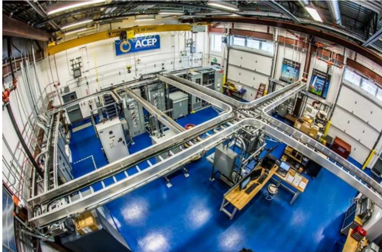
Figure 3.11. ACEP’s Power System Integration Laboratory at the University of Alaska Fairbanks is a 0.5 MW hardware-scale emulation of an isolated microgrid. Source: Alaska Center for Energy and Power, University of Alaska Fairbanks.
