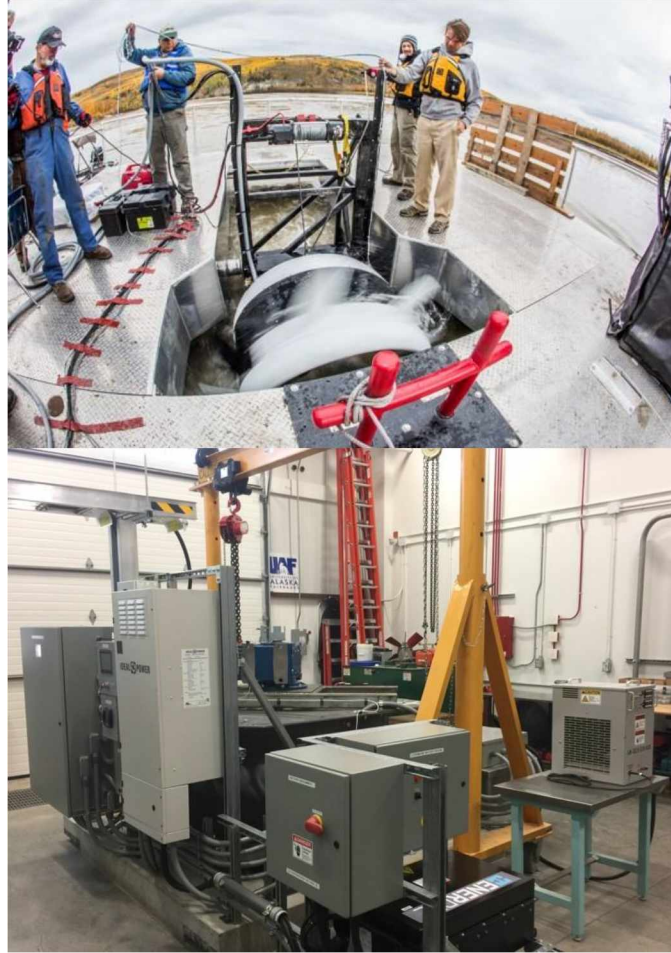
Figure 3.13. The Oceana 25 kW run-of-river hydrokinetic turbine generator during field testing (top) at the Alaska Hydrokinetics Energy Research Center’s Tanana River Hydrokinetics test site and laboratory testing (bottom) at the Power System Integration Laboratory at the University of Alaska Fairbanks. Source: Alaska Center for Energy and Power, University of Alaska Fairbanks.
