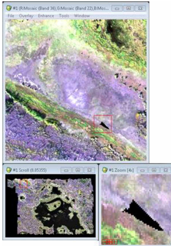
Figure 24. Example of data gap. Data gap shown in red box, and detailed in lower right window in flight area C orthomosaic introduced by masking flightline edge-pixels.
