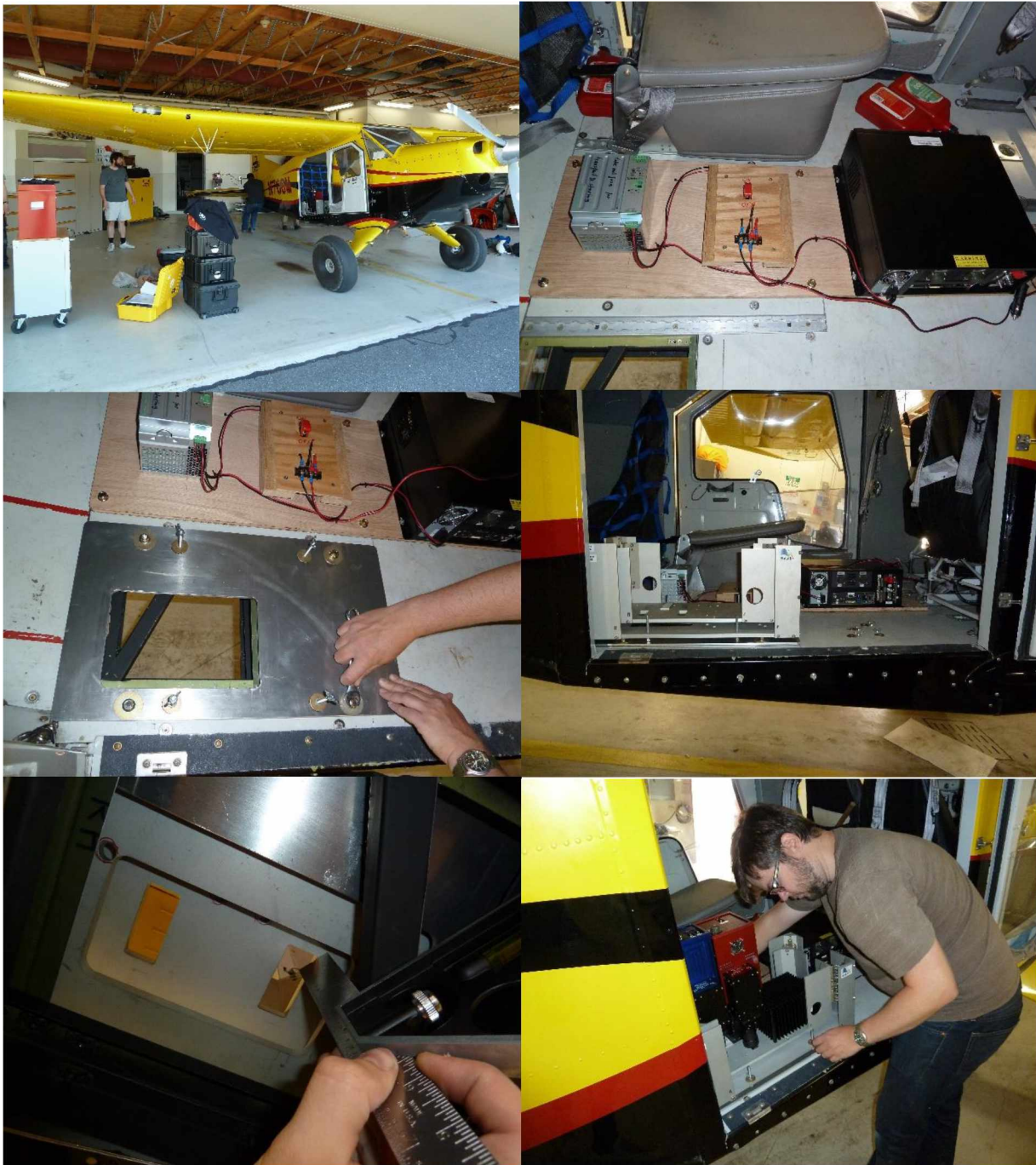
Figure 22. Mounting plates and boards. Fabrication of mounting plates and boards, and modular design of HySpex camera system allowed for rapid commissioning into aircraft, and potential for rapid deployment in subsequent acquisition campaigns
