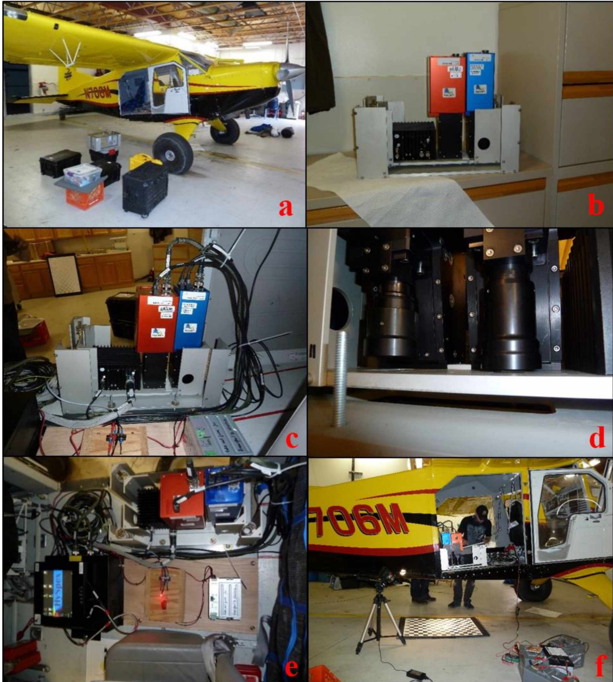
Figure 9. Commissioning the HySpex system for airborne acquisition. (a) USFWS Found Aircraft Bush Hawk; (b) VNIR-1800, Swir-384, and IMU/GPS units mounted to vibration dampening plate; (c) field of view expander optic attached to VNIR 1800 and SWIR 384 sensors; (d) detail of HySpex sensors in aircraft; (e) overhead view of the system secured and operating in aircraft; (f) testing system visibility through floor aperture of the aircraft.
