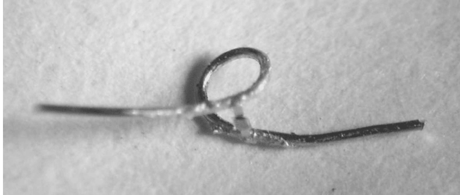
Figure 2.4: Example of loop harmonic transponder from [2]. Loop diameter is 1 mm.
