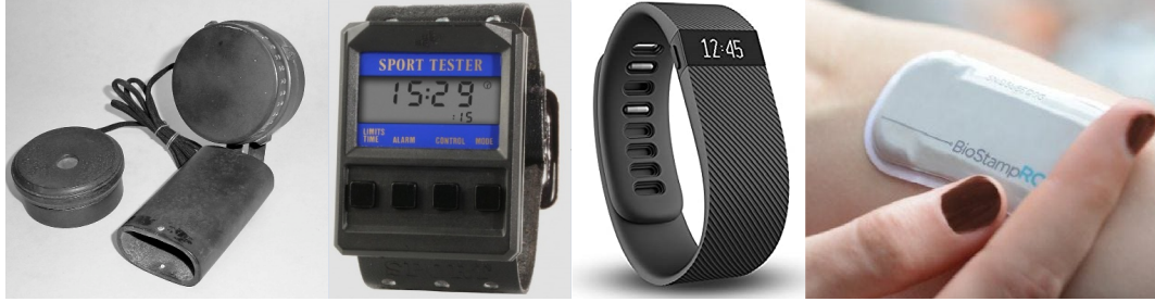
Figure 3.1: Examples of wearable devices. Left to Right: Akouphone hearing amplification device (1900), Polar Sport Tester PE 2000 (1982), Fitbit (2013), BioStamp RC (2017).
