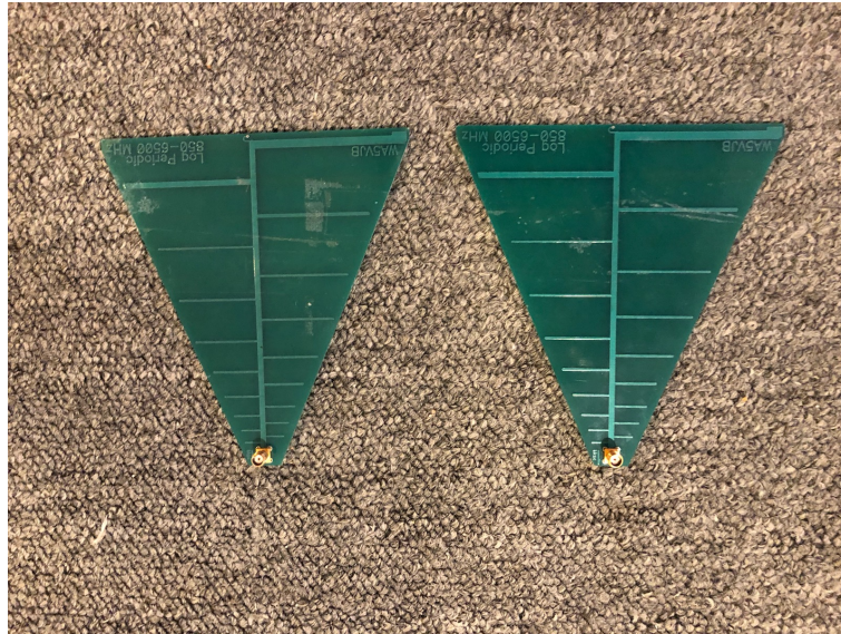
Figure 4.3: Log Periodic Antennas
