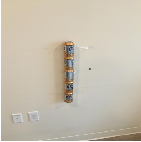
Figure 6.9: Cans to Simulate Buried Object
