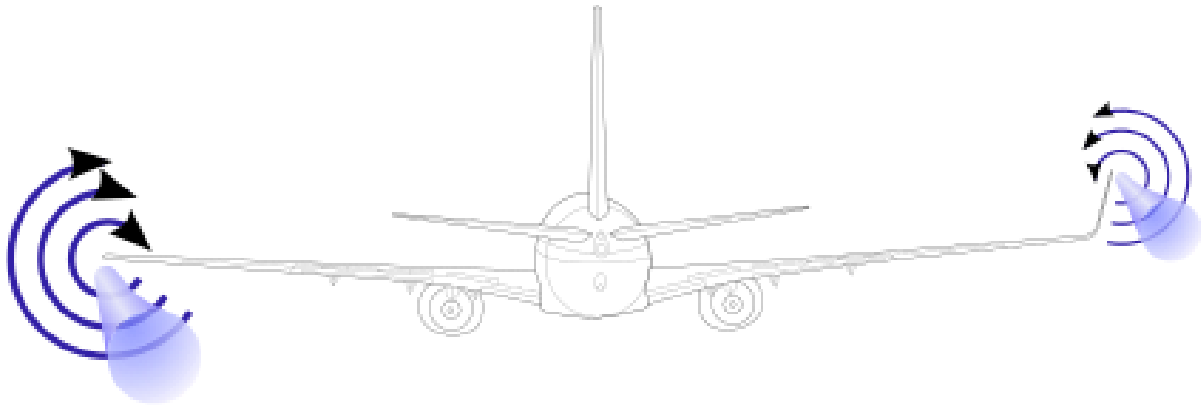
Figure 3: Effects of Adding A Winglet 9
