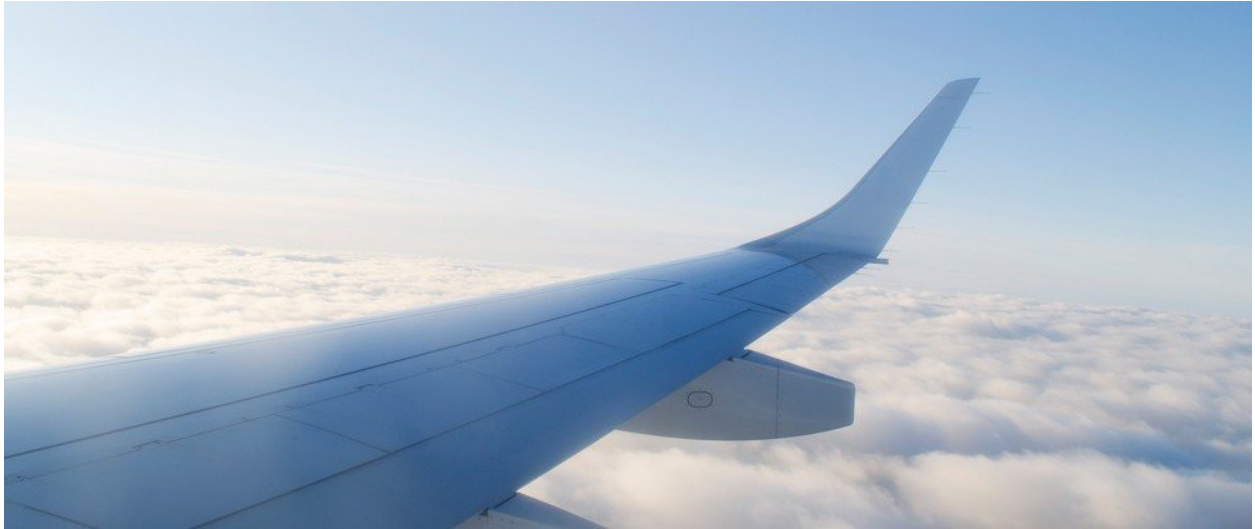
Figure 1: Example of Winglet Seen at End of Wing 3
