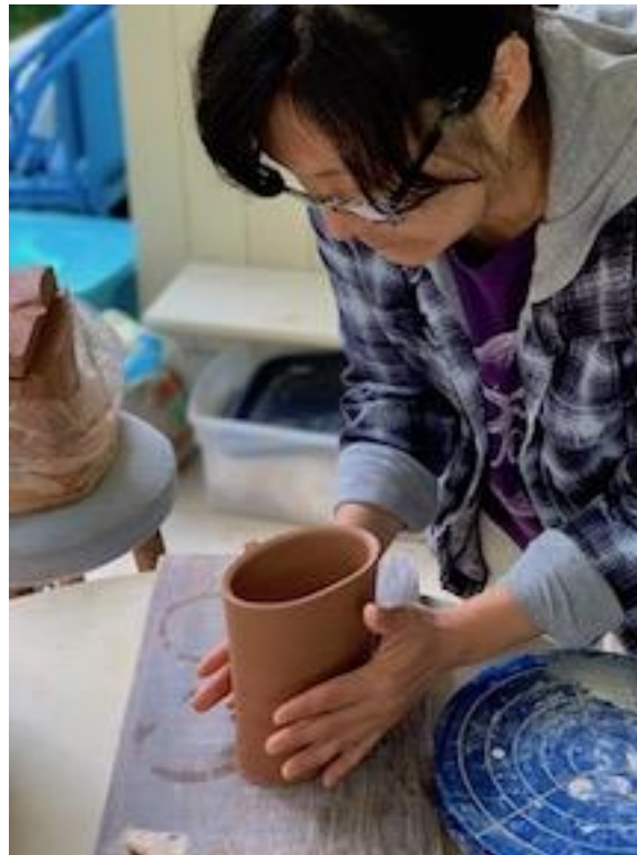
Figure F: The Process of Making a Bottle: Altering the Thrown Body
