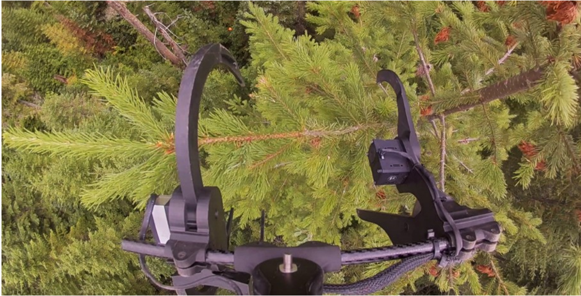
Figure 3.12 : View from the DeLeaves tool camera before collecting a branch from a 40-meter Douglas Fir.
