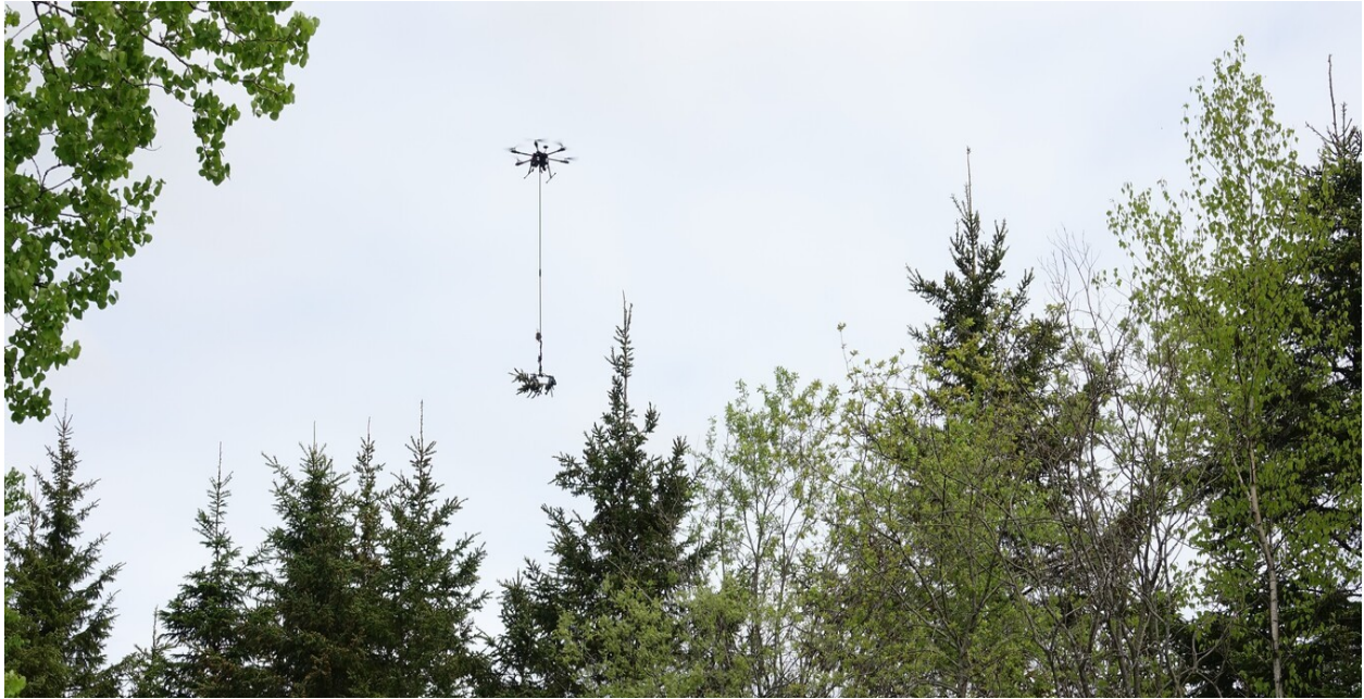
Figure 3.1 : A UAV equipped with the DeLeaves tool after collecting a red spruce ( Picea rubens ) in Quebec.
