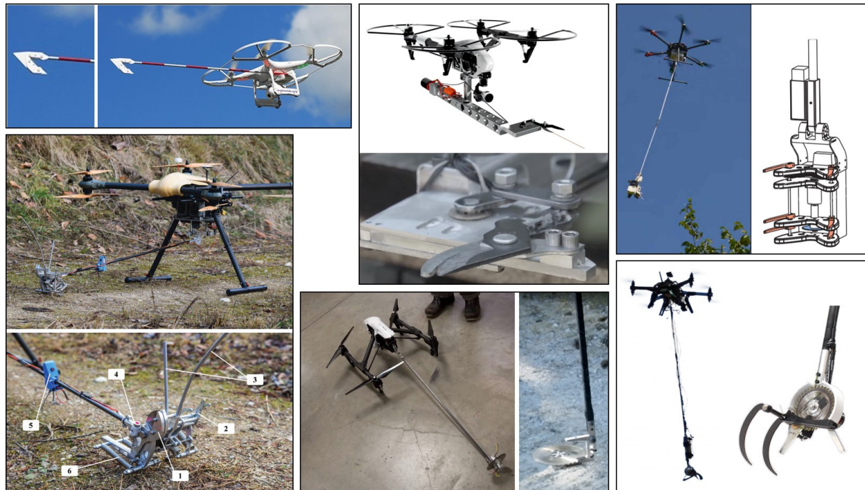
Figure 3.3 : Tree sampling UAVs from around the world. From left to right, top to bottom: UC Berkeley [16], Arborist II from Jamie Hyneman [15], FTTS from ETH Zurich [20], Lucanus from Slovenian Forestry Institute [18], Arborist I from Jamie Hyneman [14], UC Santa Barbara [17].
