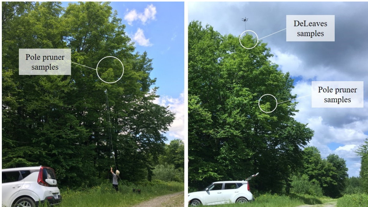
Figure 3.11 : Comparison of representative sampling locations used with CABO on sugar maples in Quebec. The pole pruner is illustrated on the left and the DeLeaves tool is on the right.
