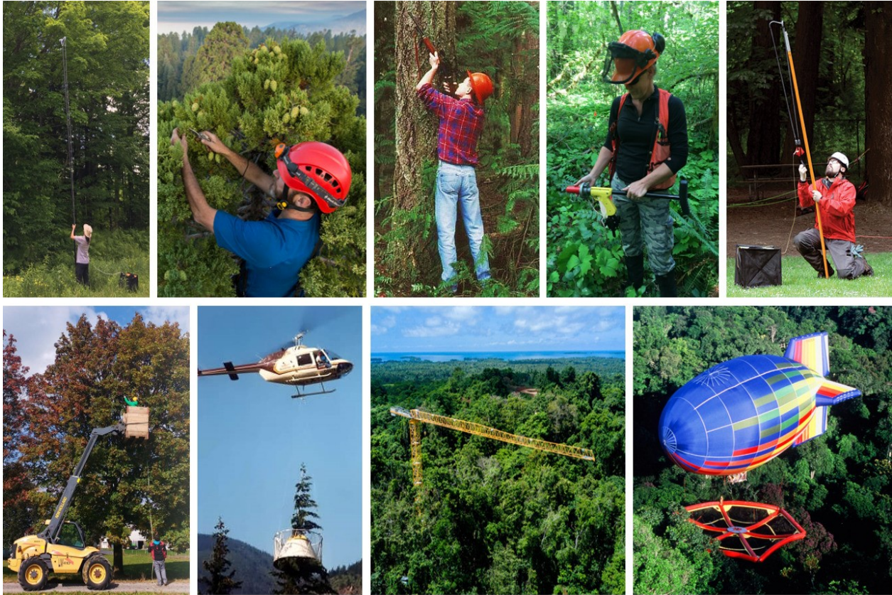
Figure 3.2 : Tree sampling techniques. From left to right, top to bottom: pole pruner, climbing [5], shot gun [4], line launchers, slingshots [50], lift [20], helicopters [4], canopy crane [48], canopy raft [7].
