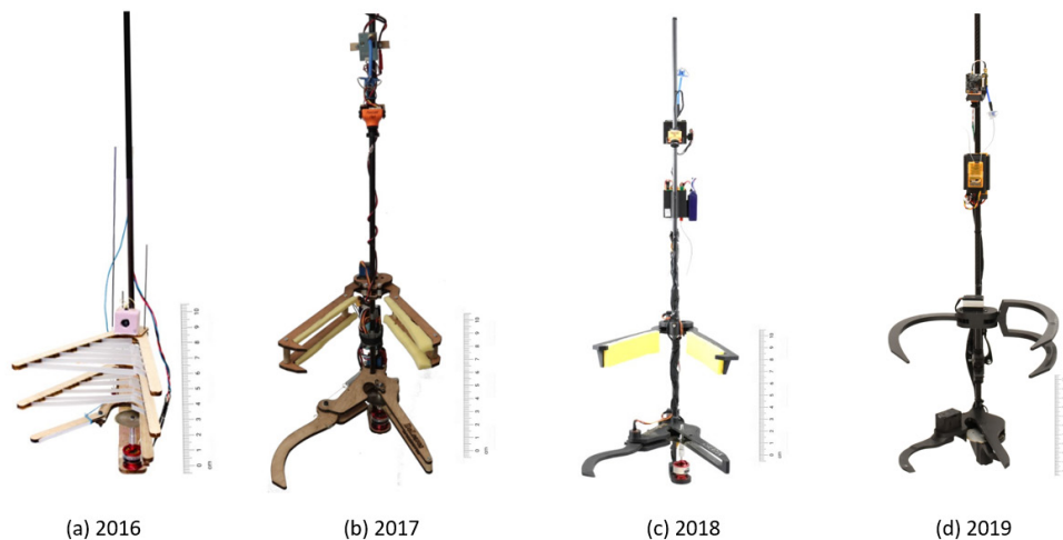
Figure 3.6 : Prototype timeline. (a) passive holding mechanism, actuated by light muscle wire, (b) servo actuated holding mechanism, grasping mechanism semi-actuated with return-spring.
