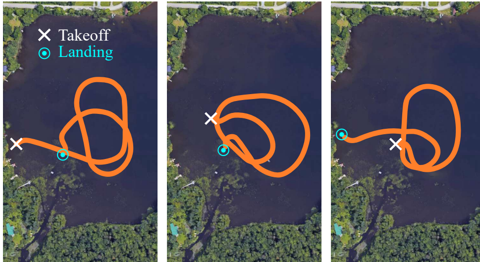
Figure 3.10 GPS tracking of three consecutive missions, with full autonomous takeoff and no physical intervention between flights.
