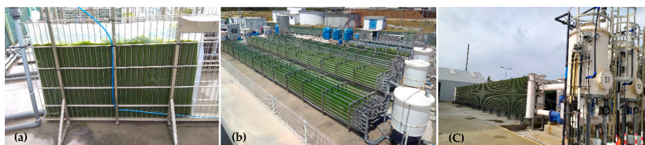
Figure 1. Different scale systems used for outdoor scale-up: (a) 0.25- \text{m}^3 flat panel photobioreactor (FP); (b) 2.5- \text{m}^3 pilot-scale tubular photobioreactor (PBR); (c) 10- \text{m}^3 industrial PBR. Pictures were provided by Allmicroalgae, Research and Development Department, Pataias, Portugal.
