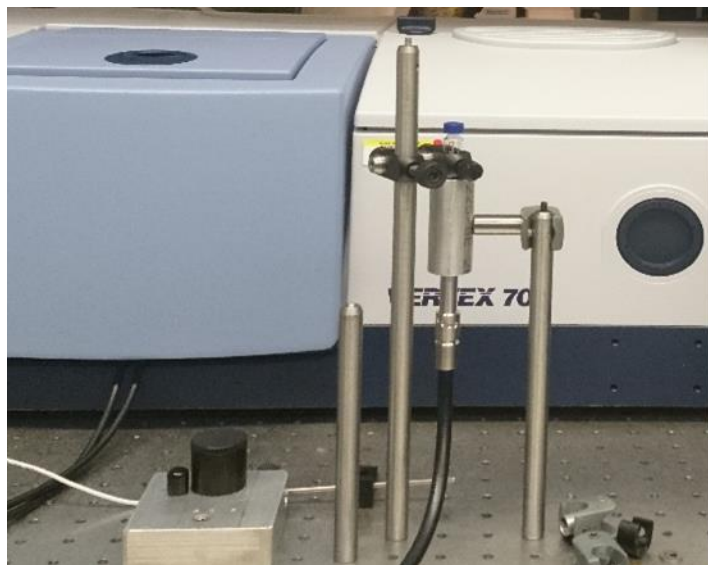
Figure 8 - Bruker® Vertex 70 FT-IR spectrometer and Spectralon (polytetrafluoroethylene, PTFE) fitted inside the HPLC vial
