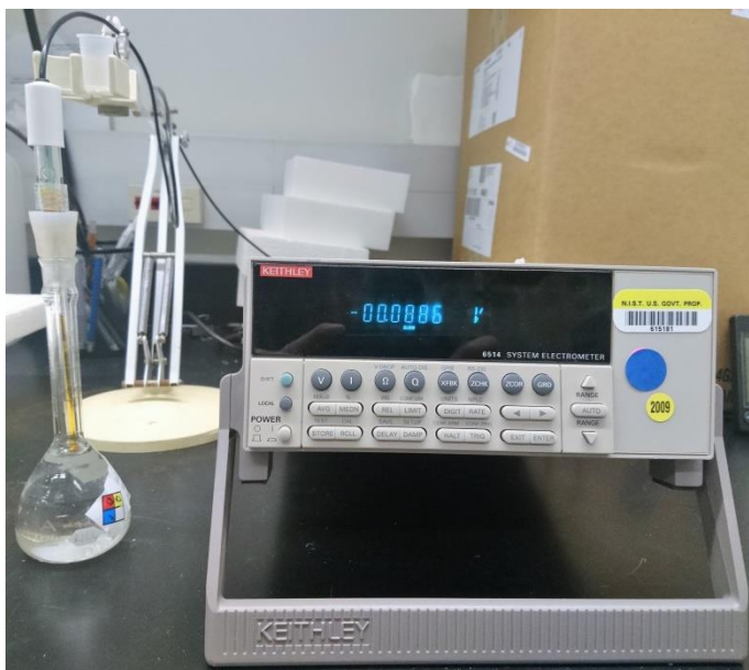
Figure 6 - Keithley model 6514 electrometer connected to a Thermo Scientific Orion Micro combination pH electrode
