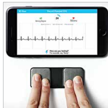
Figure. Example of a TGA-approved handheld ECG device for detecting atrial fibrillation (AF). The device is about the size of a credit card and compatible with most iOS and Android devices. Patients place their fingers on the transducer pads for 30 seconds while a one-lead ECG is recorded and transmitted to a smart phone or tablet, where it is analysed by an app with high sensitivity and specificity for detecting AF. The app provides an immediate provisional diagnosis of 'normal', 'possible AF' or 'unclassified'. 'Possible AF' should be verified by GP inspection of the rhythm strip, followed by a 12-lead ECG.
