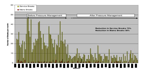
Figure 2.6 Monthly burst reductions on mains and services after pressure management (Lambert, 2010)
