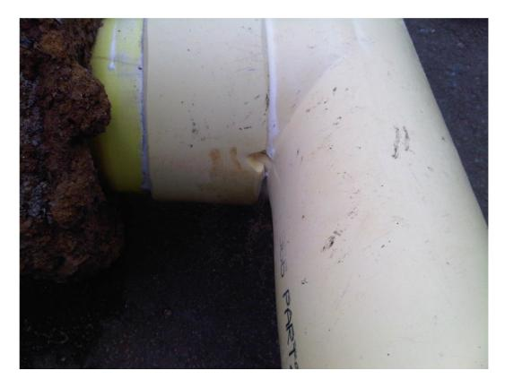
Figure D.4: Pin hole failure on a PVC tee
