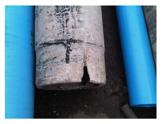
Figure D.8: AC pipe collar failure
