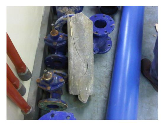
Figure D.5: Longitudinal pressure burst on an AC pipe
