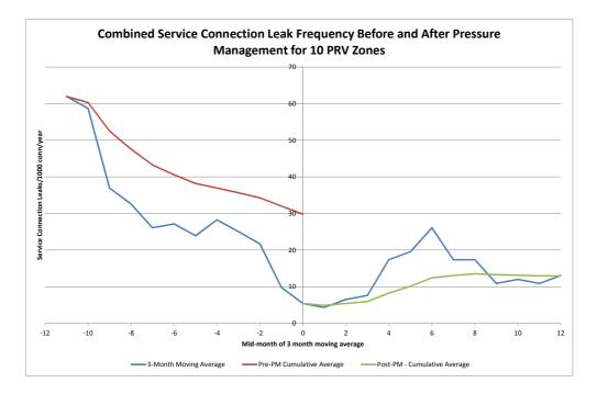
Figure 5.11: Connection Leak Frequency Before and After Pressure Management in 10 Small Zones
