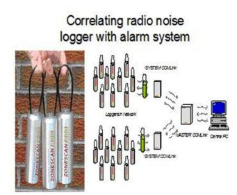
Figure 3.20: Correlating Radio Noise Logger with Alarm System. (Graphic courtesy Guttermann, 2012)
