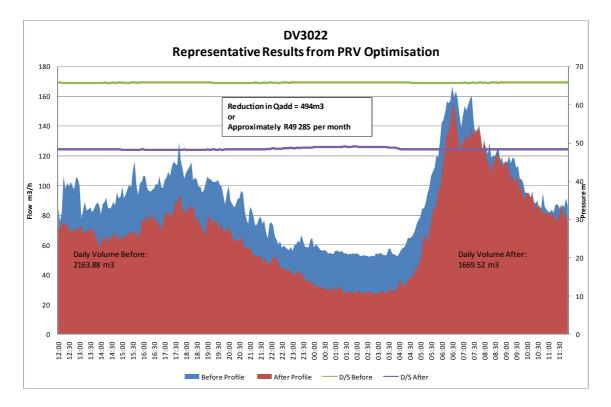
Figure 3.6: Before and After Hydrographs at DV3022
