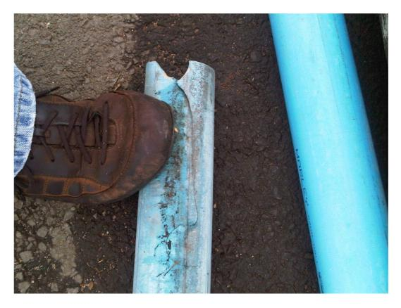
Figure D.3: Longitudinal Pressure burst on an mPVC pipe
