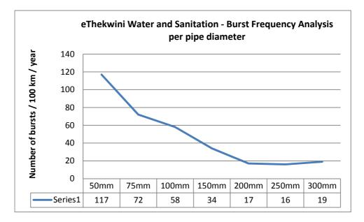
Figure 5.13: EWS Average Pipe Burst Frequency per Pipe Diameter
