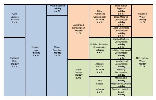
Figure A.1: The IWA Water Balance Diagram
