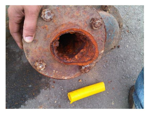
Figure D.12: Pipe failure due to corrosion at pipe wall
