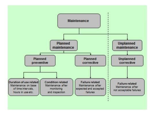
Figure 3.28: Schematic of Planned and Unplanned Maintenance (Van Der Zwan, 1989)
