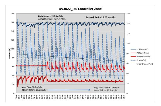
Figure 3.12: Flow and Pressure Graph with i20 Controller Fitted
