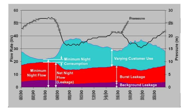
Figure 2.4: Variation of Flow and Pressure in the network (Morrison et al., 2007)
