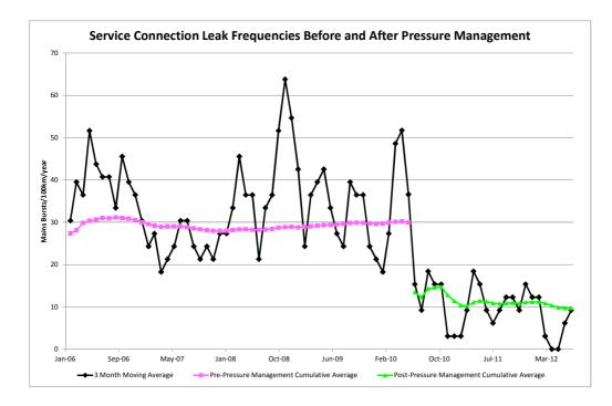
Figure 5.9: Service Connection Leak Frequency Before and After Pressure Management in the Durban CBD
