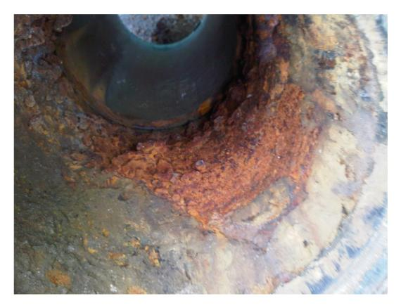
Figure D.11: Pipe tuberculation in an unlined cast iron pipe
