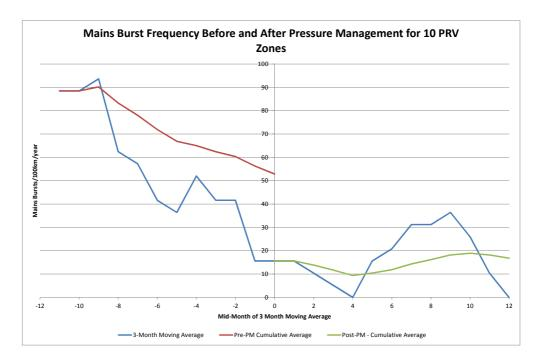
Figure 5.12: Mains Burst Frequency Before and After Pressure Management in 10 Small Zones
