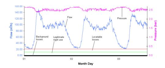
Figure 2.5: A Typical Pressure and Flow Graph from a DMA (Morrison et al., 2007)
