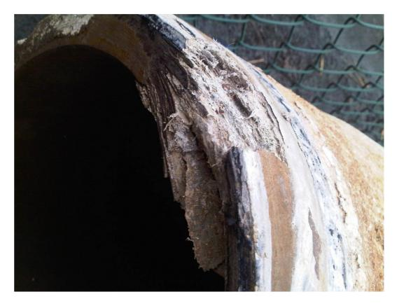
Figure D.9 AC pipe degraded through soft water attack
