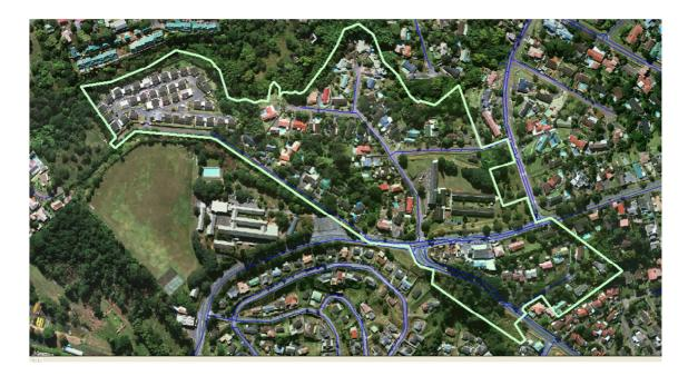
Figure 3.5. A new PRV Zone in Northdene, Durban
