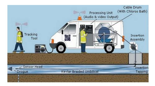
Figure 3.23: An example of In-pipe Acoustic Technology (SSIS Consulting Engineers, 2010)
