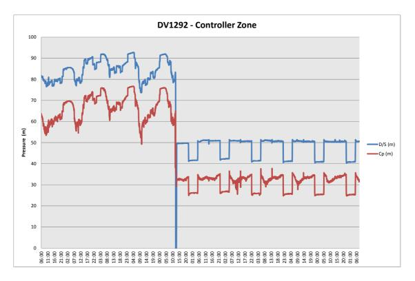
Figure 3.8: Pressure Profile at DV 1292 with time controller fitted
