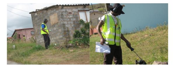
Figure 3.16: Mechanical Leak Detection using amplified listening stick. (Photo courtesy of Mr Chris Otto, 2010)
