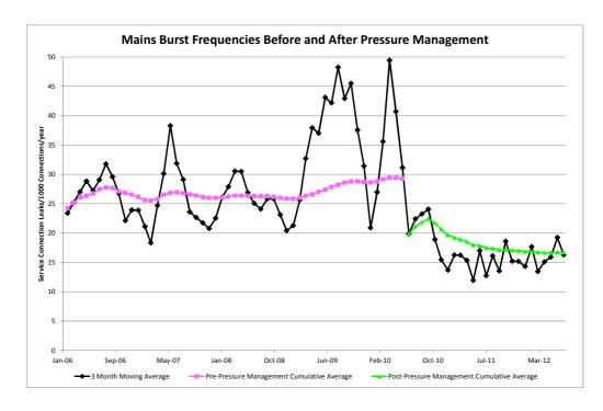
Figure 5.10: Mains Burst Frequency Before and After Pressure Management in the Durban CBD
