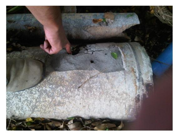
Figure D.7: Hole failure in an AC pipe
