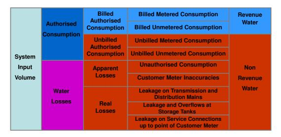
Figure 2.7: The IWA Water Balance (Lambert et al., 2000)
