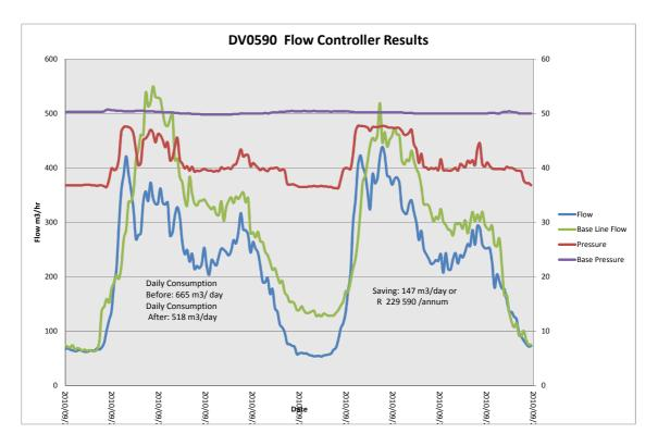
Figure 3.11: Flow and Pressure Graph with Flow Controller Fitted
