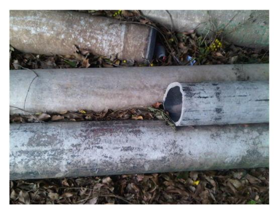
Figure D.6: Ring fracture on an AC pipe caused by settlement
