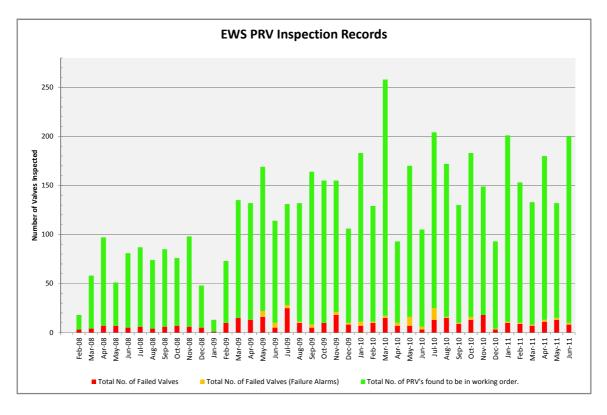
Figure 3.2: Results of PRV Inspections
