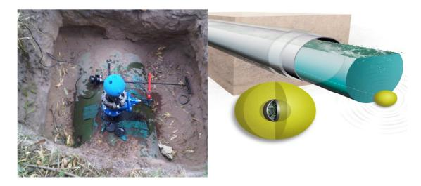
Figure 3.24: Smart Ball Internal Noise/Leak Technology (SSIS Consulting Engineers, 2010)
