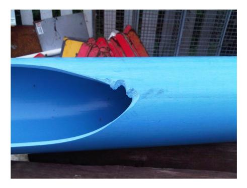
Figure D.2: Pressure burst on a mPVC main
