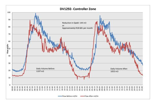
Figure 3.9: Flow Profile at DV 1292 with time controller fitted
