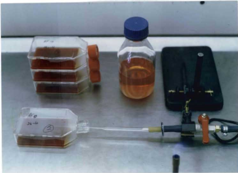
Fig. 3. Culture system, tissue-culture flasks being gassed with a mixture of 3% O 2 , 4% CO 2 and 93% N 2 .
