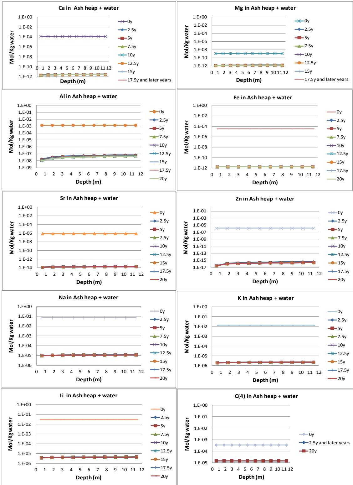
Figure 5.6: Total elemental concentration of major and minor elements in the leachate, against the depth at certain years of ash heap irrigation with water
