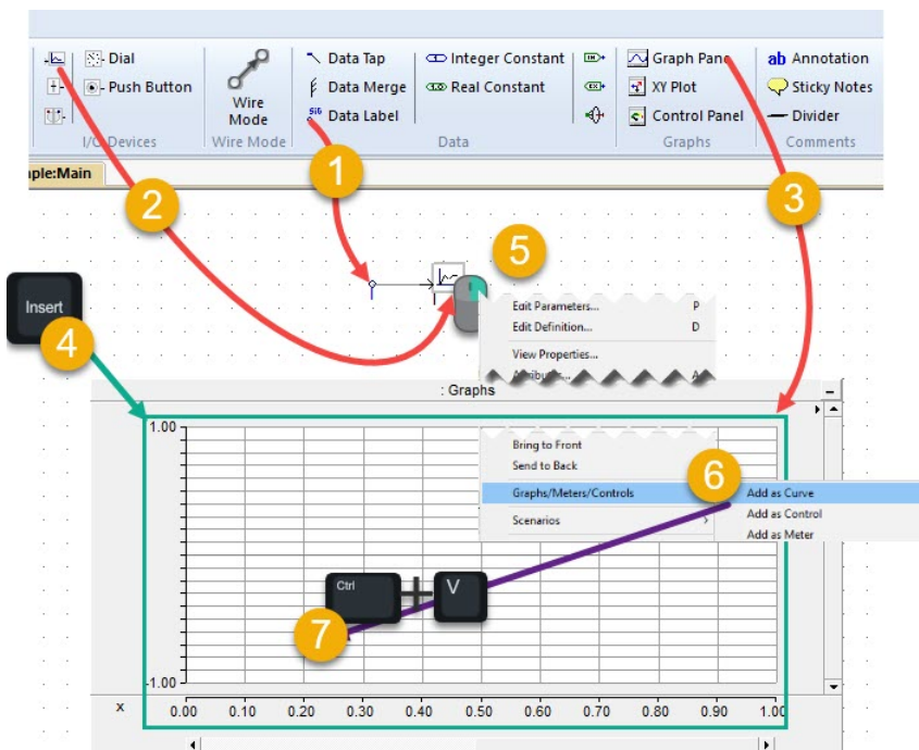
Figure B.14: How to set up an output channel and a plot
