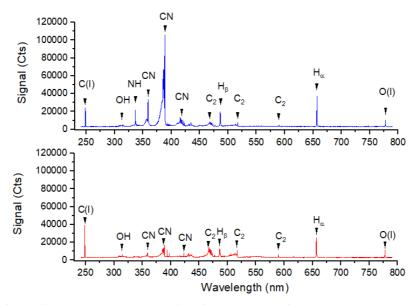
Fig.1 Ribose LIBS spectra acquired in (top panel) air atmosphere and (bottom panel) Martian atmosphere.
