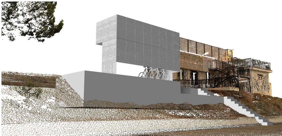
Figure 3. 3d rendering of the prototype implemented on a 3D laser scan of the site
