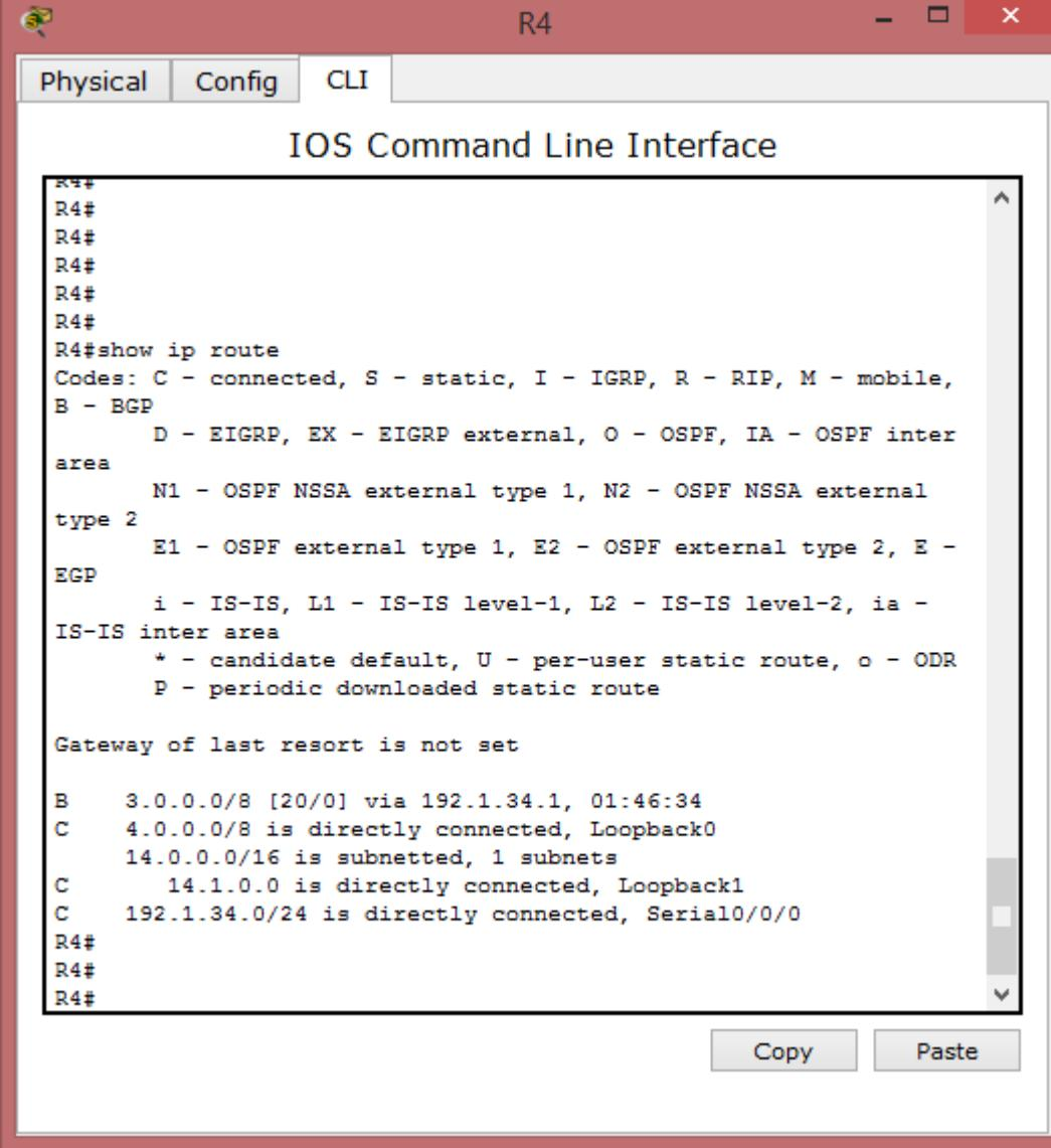
The screenshot shows a Windows Command Line Interface window titled "R4". The window has tabs at the top: "Physical", "Config", and "CLI". The "CLI" tab is selected. Below the tabs is the title "IOS Command Line Interface". The main area of the window displays the output of the "show ip route" command. The output includes a legend for route codes and a list of routes.
