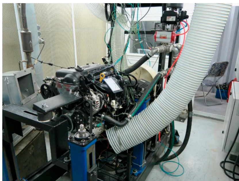
Figure 1. Experimental testing of KIA Cerato engine on engine test bed.
