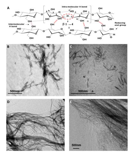
**Figure 1.** Cellulose structure and intra/intermolecular hydrogen bonding pattern (**A**). Morphological and structural characteristics of the unmodified and oxidised nanocellulose samples: Transmission electron micrographs of cellulose nanocrystals (**B**), oxidised cellulose nanocrystals (**C**), cellulose nanofibers (**D**) and oxidised cellulose nanofibers (**E**). Reprinted with permission from Tayeb et al. [30] and Siqueira et al. [31].
