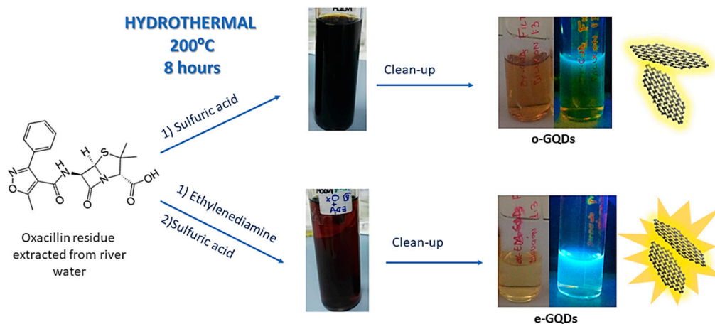
Figure 1. Schematic representation of the synthetic procedure of graphene nanostructures from oxacillin residues recovered from water samples. Pictures of graphene quantum dot (GQD) dispersions in water under sunlight ( left ) and UV lamp ( right ) irradiation are shown.
