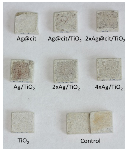
339 Fig. 7. Digital photographs of limestone slabs after the application of treatments (200 \mu L of an aqueous 340 suspension of nanocomposites). All of the silver-bearing treatments have the same silver dose.
