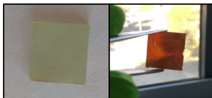
Figure 3.12. (Left) White solid formed on the substrate when the antisolvent is not added during the spin-coating step. (Right) MAPbI 3 perovskite film fabricated at ambient conditions.
