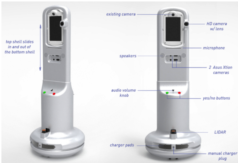
Figure 7.2: Final disposition of sensors on TERESA. The sensors used for navigation are the LIDARs (there is another one in the back, not shown here) and the XTion cameras.
