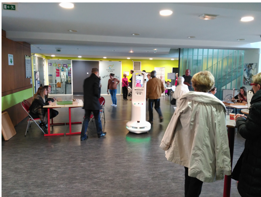
Figure 7.1: Image of the telepresence robot developed in the TERESA project navigating among people.
