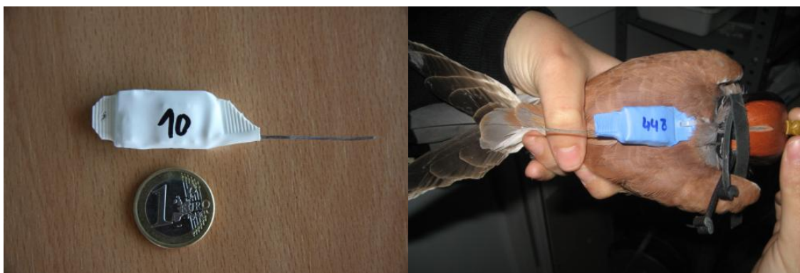
Figure 5. GPS-datalogger with thermoretractable case. Detailed view of the device in comparison to a coin (left panel) and of its deployment on an individual lesser kestrel back (right panel).
