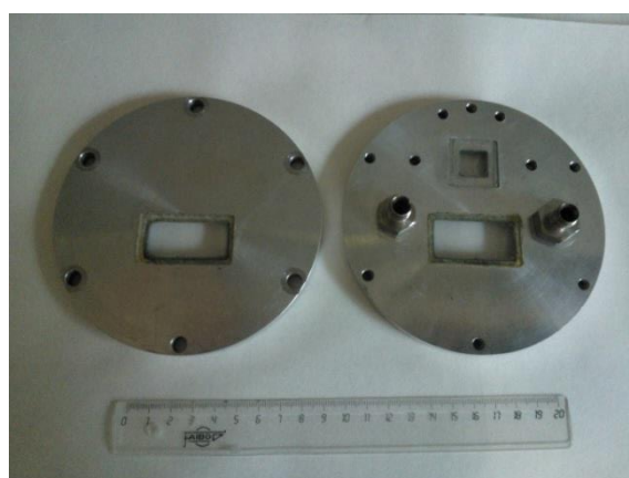
Figure 2.6.- Outer view of gas testing chamber. Left, back of the chamber, right, front of the chamber. In the front of the chamber are the inlet and outlet of gases.
