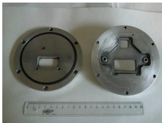
Figure 2.5.- Inner view of the gas testing chamber. Left, a window for UV-Vis spectroscopy, right, two windows for UV-Vis and Fluorescence combined spectroscopies.
