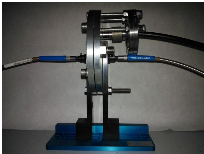
Figure 2.7.- Gas sensor chamber. The different optical fibers are placed in the chamber. The metallic and blue fibers are for UV-Vis spectroscopy and the black fiber is for fluorescence spectroscopy.
