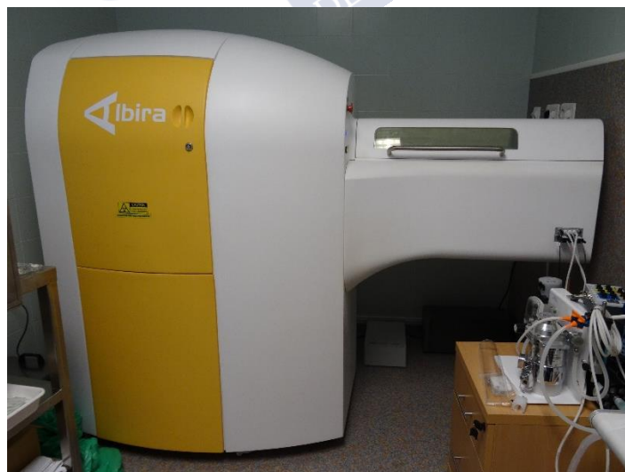
Figure 6. Image of a micro-PET/CT small animal imaging system (Albira PET/CT Preclinical Imaging System, Bruker Biospin, EEUU).
