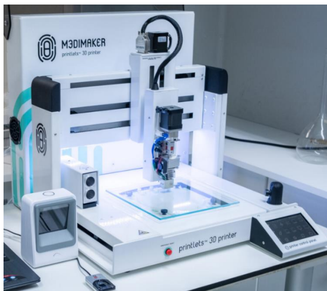
Figure 8. Image of a 3D printer suitable for the manufacture of pharmaceutical products (M3DIMAKER™, FabRx Ltd., UK).
