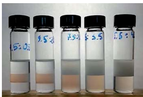
Figure 4.3. Blend scan for IGEPAL CO-520/ [\text{C}_6\text{mim}][\text{OAc}] at 298.15 K and 2 %wt salt
