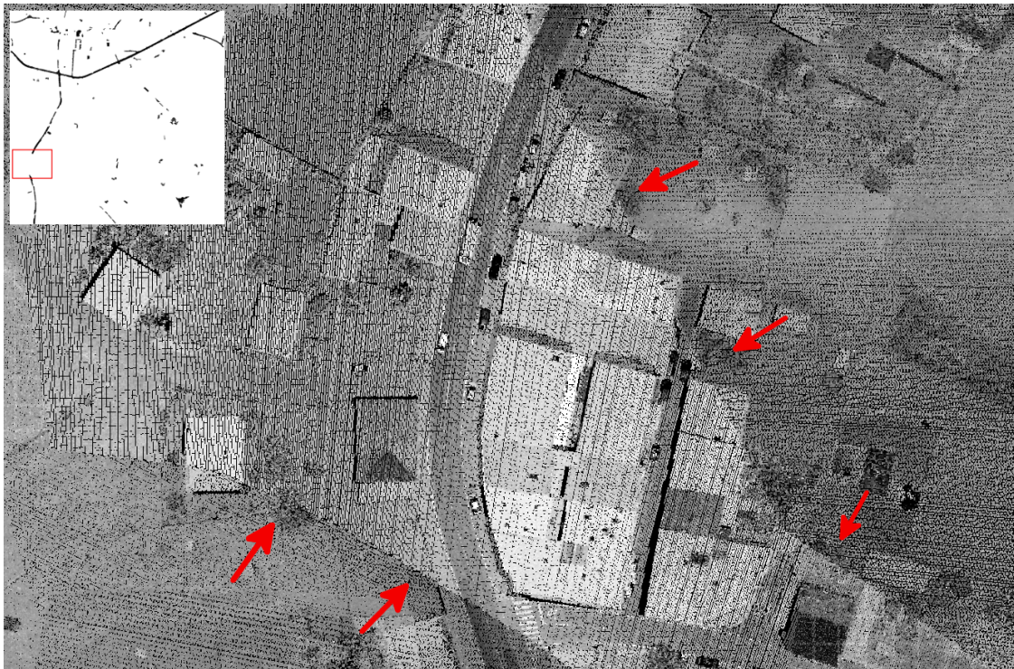
Figure 12. Intensity correction issues in Arzúa. The change in intensity is clearly visible at the overlap of the flight strips (highlighted with red arrows). The road segment inside this high-intensity strip cannot be identified by our method because of its high intensity compared with other road segments.
