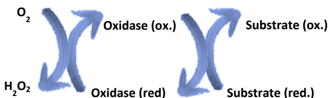
Figure 1.2. Oxidation mechanism of oxidases
