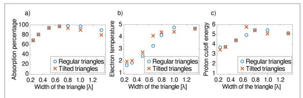
**Figure 5.** (a) Laser energy absorption percentage, (b) electron temperature and (c) proton cutoff energy as a function of the structure width. The height of the structures is  $h=\lambda$ . The electron temperature and proton energy are normalized to the values obtained for a flat target.
