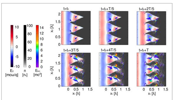
**Figure 1.** Illustration of the electron dynamics over a laser period T, taken from a PIC simulation, with six snapshots of the electron density, the  $E_2$  component of the electric field, in which the laser field is polarized, and the most energetic electrons, colored depending on their kinetic energy. The electrons move in the vacuum gap from one triangle to the next according the sign of the  $E_2$  component of the electromagnetic field, gaining energy in the process.
