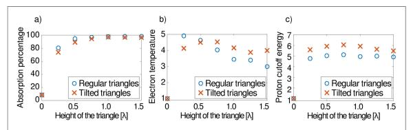
**Figure 6.** (a) Laser energy absorption percentage, (b) electron temperature and (c) proton cutoff energy as a function of a structure height. The width of the structures is  $w = 0.7\lambda$ . The electron temperature and proton energy are normalized to the values obtained for a flat target.
