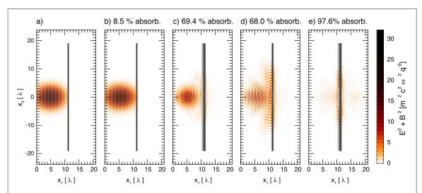
**Figure 4.** (a) Incident and (b)–(e) reflected electromagnetic energy density for different structured targets. The reflected field is shown for a (b) flat target and targets with structure height and width of: (c)  $h = \lambda$  and  $w = 0.25\lambda$ , (d)  $h = 0.25\lambda$  and  $w = \lambda$  and (e)  $h = \lambda$  and  $w = 0.7\lambda$ .
