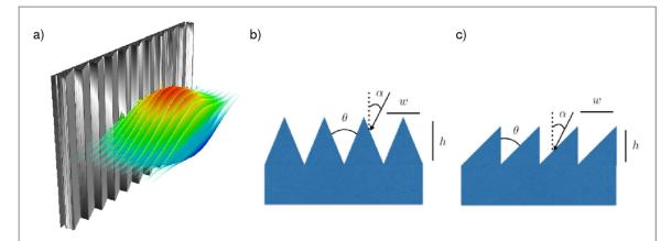
**Figure 3.** Shapes of the triangular structures. (a) 3D image of the simulation setup and (b), (c) detailed view of the 2D targets. The variable h represents structure height, w the width,  $\theta$  the angle formed between two neighboring structures and  $\alpha$  the angle of lase incidence towards the target.
