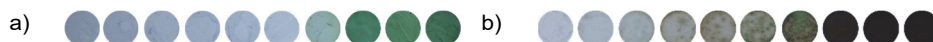
Fig. 2. Sensory response of F1a discs to: a) chlorine, [\text{Cl}_2] : blank, 16, 39, 79, 118, 157, 394, 787, 1180 and 1574 ppbv; b) hydrogen peroxide, [\text{H}_2\text{O}_2] : blank, 34, 87, 174, 261, 347, 868, 1737, 2605 and 3474 ppbv.
