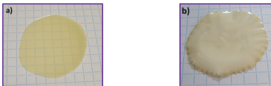
Fig. S1. Photographs of the aramid film with 50 % of IL. a) Before the removal of the IL; b) After removing the IL in distilled water during 24 h.
