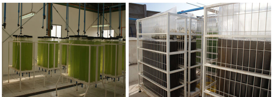
FIGURE 1 Images of the culture systems used in our experiments. Left: the bubble-column reactors used at laboratory scale; Right: the flat-panel reactors used outdoors [Colour figure can be viewed at wileyonlinelibrary.com ]
