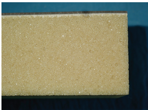
Fig. 3: Shows one of the polyurethane blocks used in the study, where the imitation of cortical and trabecular bone can be observed.
