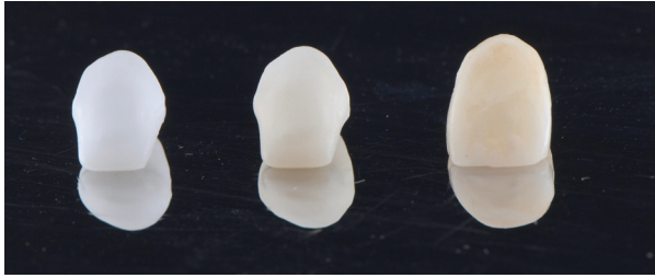
Fig. 1: Color measurement of colored Zr core on white background and color measurement of white Zr core on black background.
