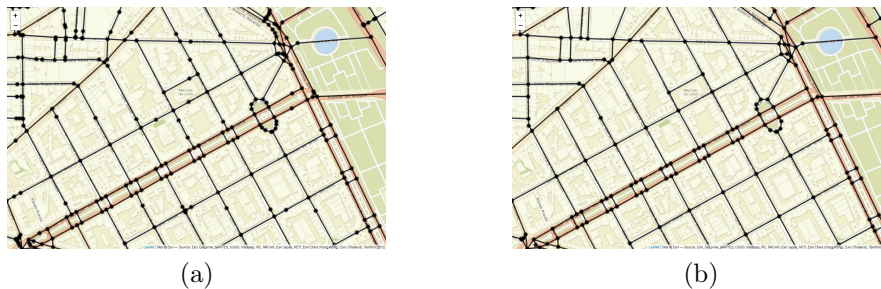
Figure 8.5: A road network introduced as input (a) and its simplified version after the application of the SimplifyLinearNetwork function with Angle = 25 and Length = 65 (b)
