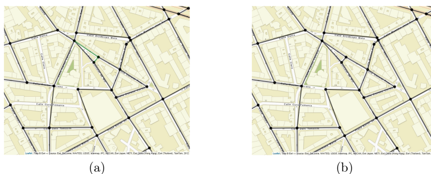
Figure 8.4: Another use of the "Join vertex" (in green) option of the "Network Edition" section (a) that leads to the final corrected road structure in (b)
