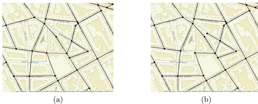
Figure 8.3: Use of the "Join vertex" (in green), "Remove edge" (in red) and "Add point" options (in green) in the SpNetPrep application (a), and resulting network after pressing "Rebuild linear network" (b)
