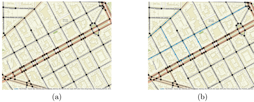
Figure 8.6: A zone of a road network introduced as an input in the "Network Direction" section of the SpNetPrep application (a) and manual addition of traffic flow to the network by using the options "Add flow" and "Add long flow" (b)
