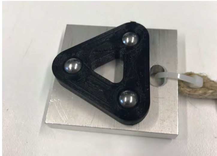
Figure 11.4: The designed ball bearing to reduce constraint forces
