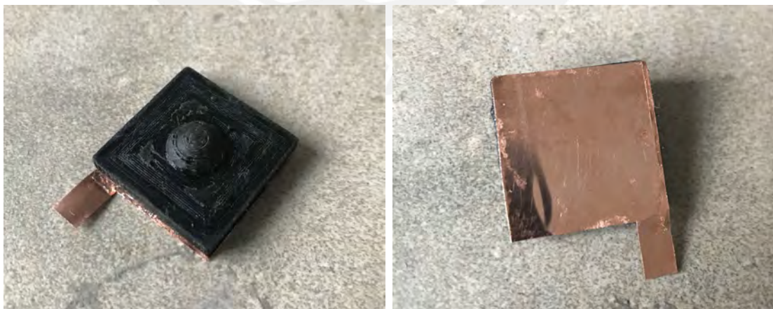
Figure 10.1: The force transducer with copper plate, top and bottom view
