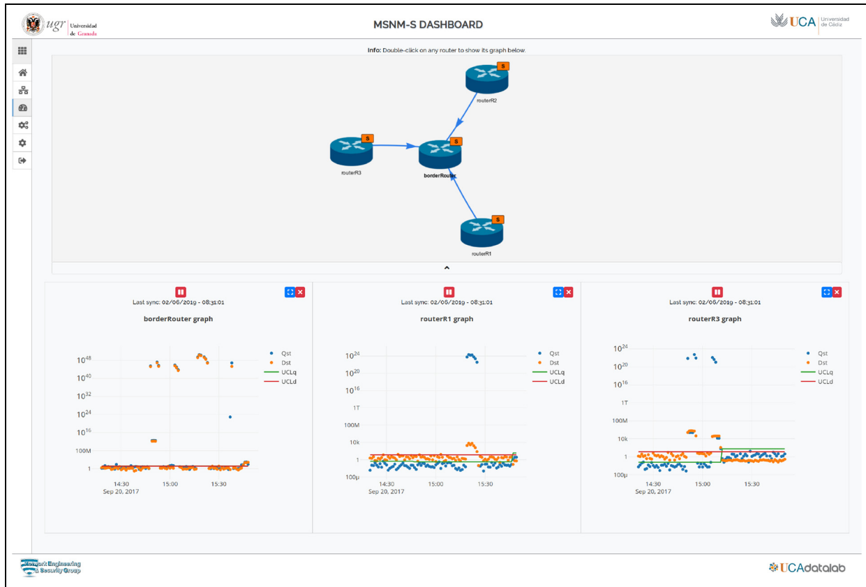
Figure 5. Snapshot of the monitoring view of the MSNM-Sensor dashboard. The logical connections of the sensors (orange boxes) are shown in the upper section of the figure, while the monitoring graphs are in the bottom part.
