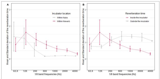
**FIGURE 3 | (A)** Average reverberation time within the incubator in the reverberant (Nreverb, *pink*) and absorbent (Nabs, *gray*) rooms. **(B)** Reverberation time inside (*pink*) and outside (*gray*) the incubator in the reverberant room Nreverb.
