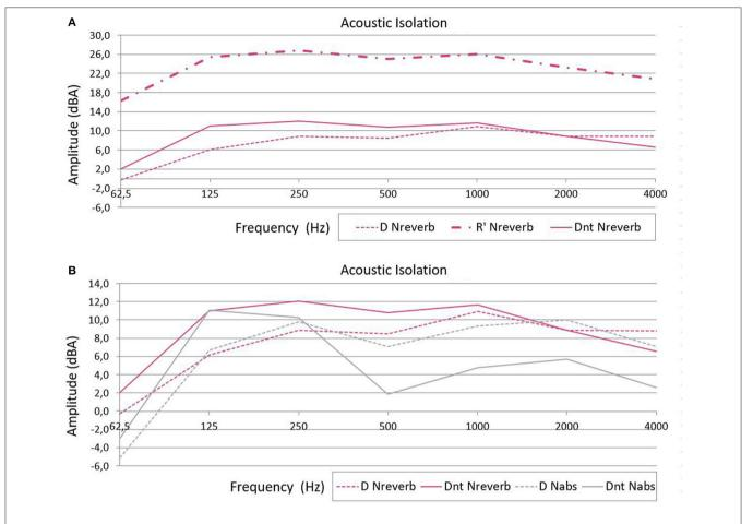
FIGURE 2 | (A) Level difference (D), apparent sound reduction index (R'), and standardized level difference (DnT) isolation indexes (in dBA) for the incubator in the reverberant room. (B) Comparison of the level difference (D) and standardized level difference (DnT) isolation indexes of the acoustic absorbent (Nabs, gray) and reverberant (Nreverb, pink) rooms.
